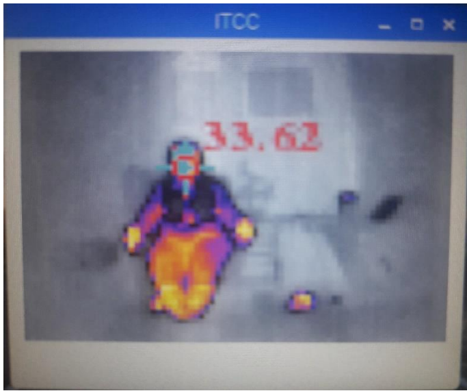
Fig. 7 Skin temperature measured with the system.
